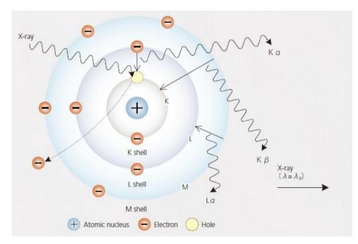
Figure 2.1 Electron Paths and Principle of X-ray Generation Expressed as a Bohr Model
